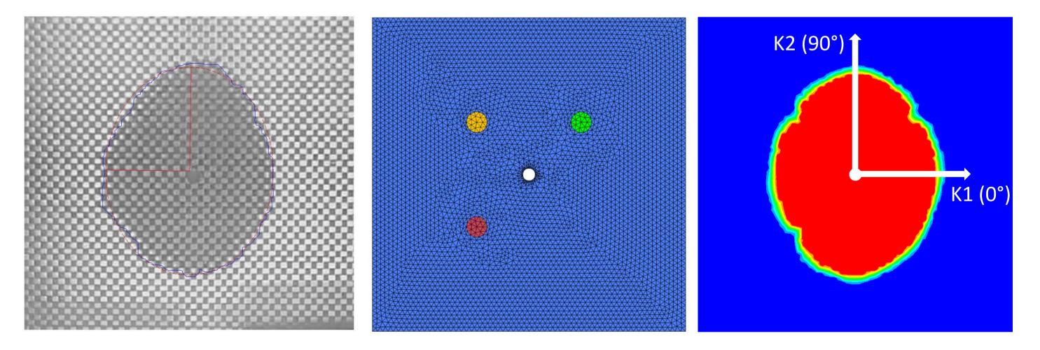
**Figure 3**: Test view (left), fabric layer with resistive welding zones (green, yellow, red) (middle), numerical flow front (right)
